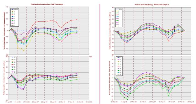
The red line (Station 7 - Oak - top left-hand graph) suggest there was a persistent deficit through the winter of 2006 which has since replenished itself. Total movement for the Oak is 40mm and for the Willow, 60mm. The soil beneath the Oak is a heterogeneous mixture with pockets of sands and gravels whereas the soil beneath the Willow is a more consistent clay.
